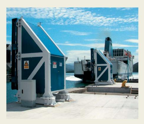
Thanks to the innovative MoorMaster design the mooring of a ship can be done in a fraction of the time and cost compared to mooring with ropes.
